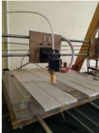
Figure 6: Shaft being 3-D Printed
