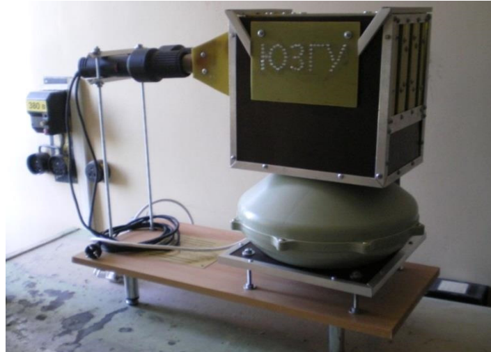
Figure 2. Scheme of the experimental setup. 1 – housing; 2 – pipe for the inlet of the heating medium; 3 – construction Hairdryer; 4 – axial fan; 5 – stand for the fan; 6 – LEDs.
