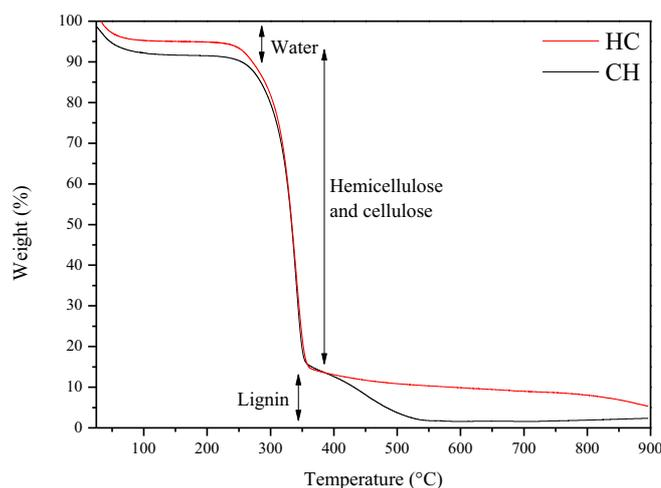
**Figure 6.** TG curve with mixed reagent.
