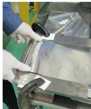
Figure 3. Photograph of manual jelly rolling.
