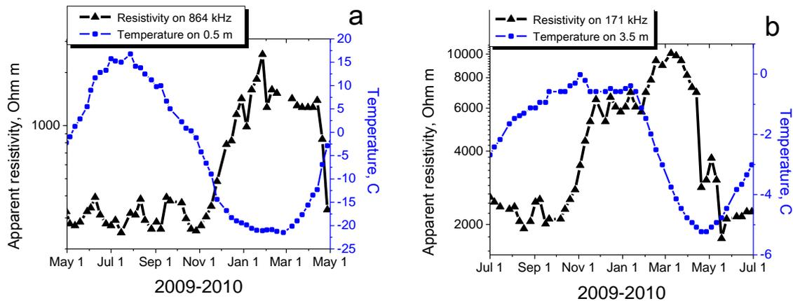
**Figure 1.** Seasonal temperature variations at depths of 0.5 m (AL) and 3.5 m (LATF) compared to seasonal variations of apparent resistivity at frequencies of 864 and 171 kHz, respectively.
