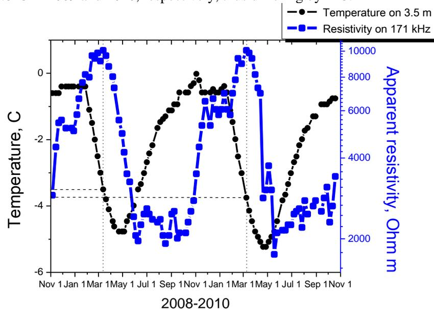
**Figure 3.** Seasonal variations in ground temperature at 3.5 m depth and apparent resistivity at 171 kHz frequency in 2008-2010.
