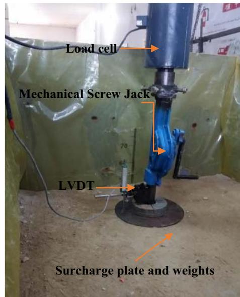
**Figure 5.** apparatuses of in-situ CBR test.
