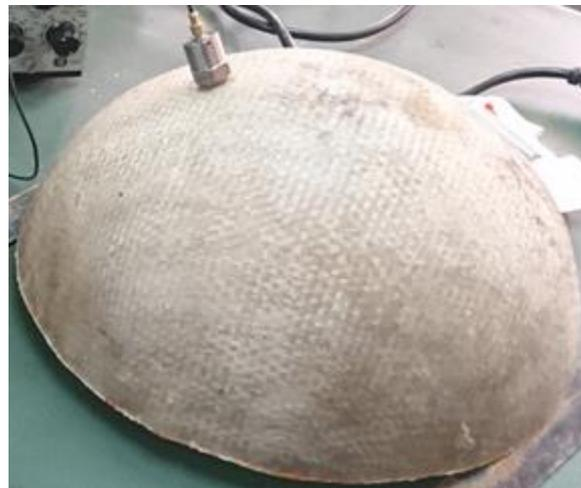
**Figure 2.** Manufacturing the orthotropic spherical composite shell cap
