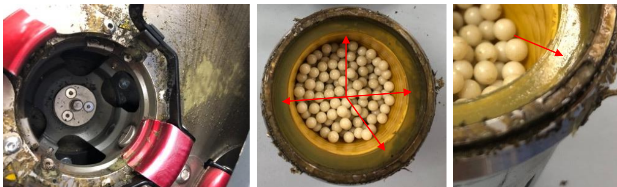
Figure 8. Sample burn out and escape from milling bowl.
