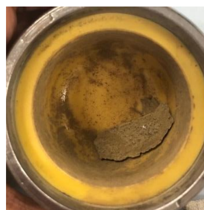
Figure 5. Dry method grinding of rice husk.
