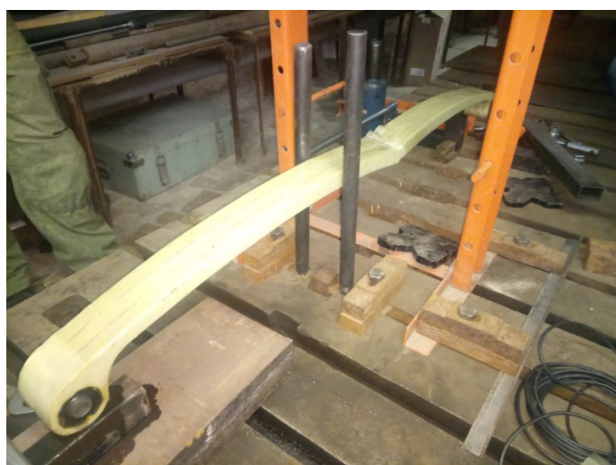
Figure 6. The leaf spring is destroyed
