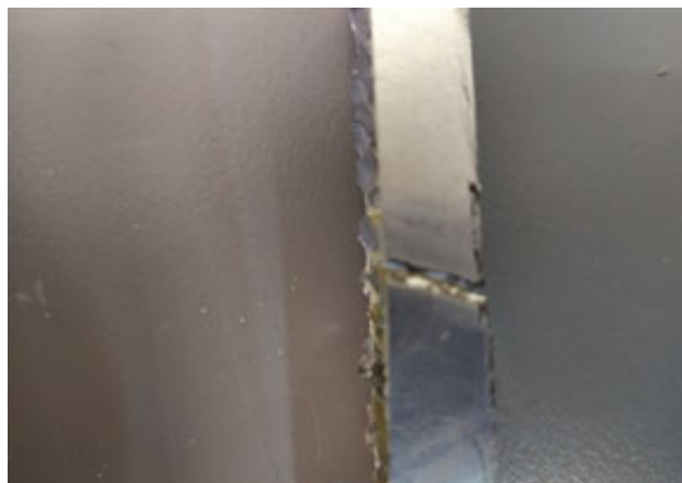
Figure 7. View of a specimen after a tensile test at -70 °C.
