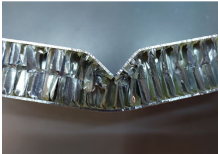
Figure 16. View of a specimen after a three point bending test at -70 °C.
