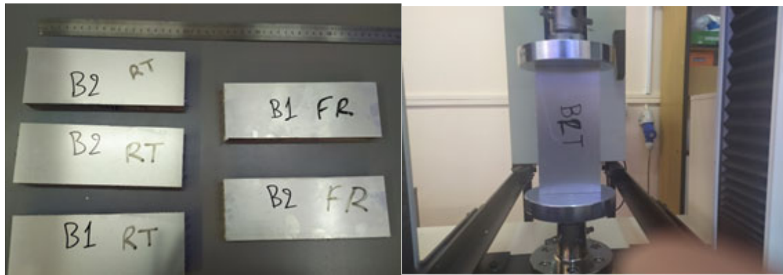
Figure 3. a) Specimens for edgewise compression b) Edgewise compression testing in aluminum sandwich specimen.
