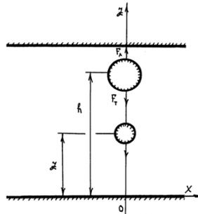
**Figure 1.** The settling dust process model in a limited production volume
