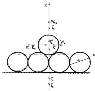
**Figure 2.** Model of the raising dust process from the surface
