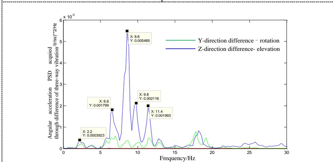
**Figure 17.** Angular velocity PSD spectral line of packaging box baseplate.
