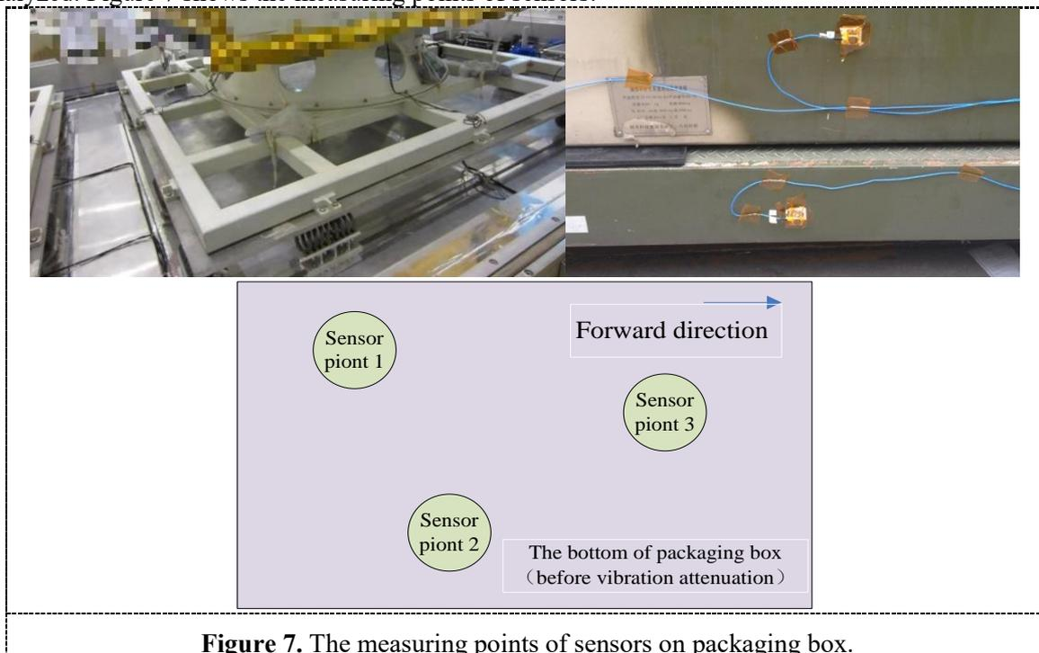
**Figure 7.** The measuring points of sensors on packaging box.
