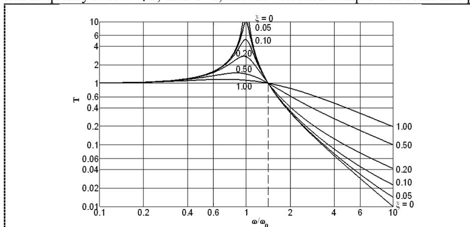
**Figure 2.** Reelationship between transmissibility, frequency and damping.
