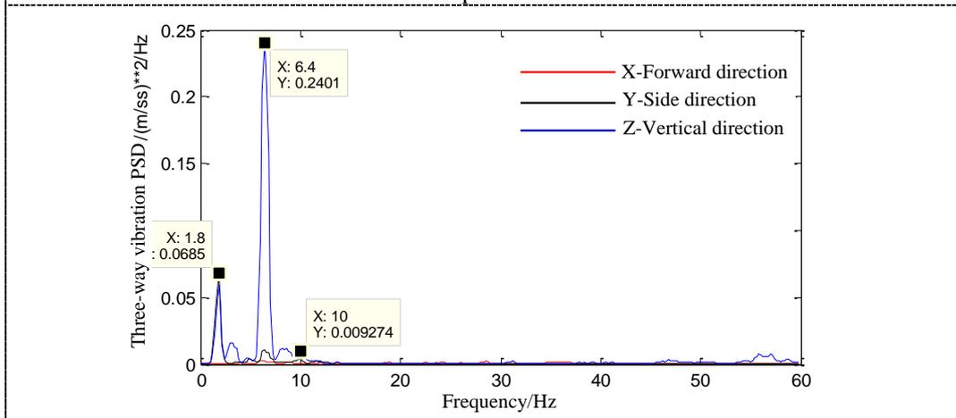
**Figure 16.** Vibration acceleration PSD spectral line of measure point 1 during railway transportation.
