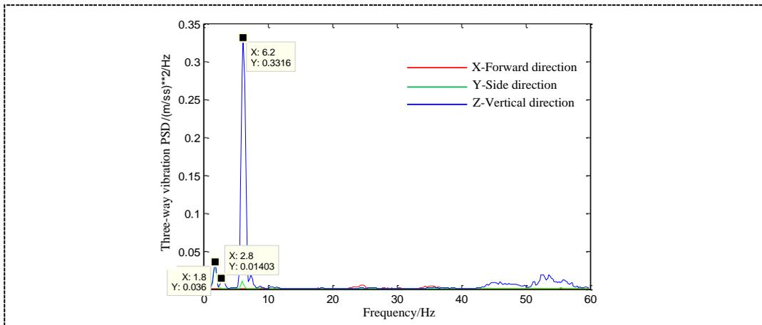
**Figure 15.** Vibration acceleration PSD spectral line of measure point 1 during railway transportation.
