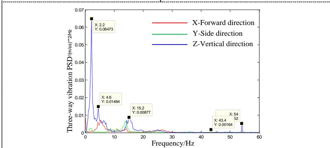
**Figure 11.** Vibration acceleration PSD spectral line of measure point 2 during highway transportation.
