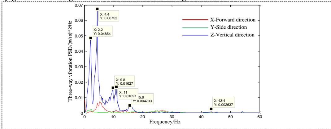
**Figure 10.** Vibration acceleration PSD spectral line of measure point 1 during highway transportation.
