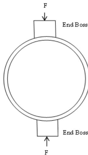
**Figure 1.** Ring Shape Force sensor
