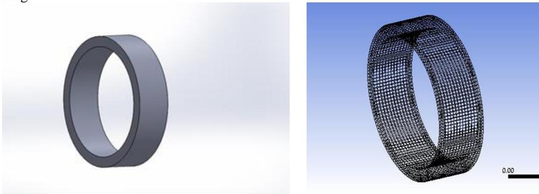
**Figure 2.** CAD modeling of elastic ring sensor with meshing
