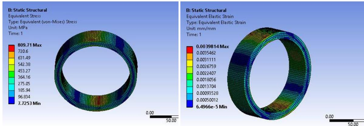
**Figure 3.** Stress and Strain variation in ring transducer (50kN)
