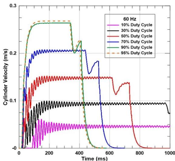
**Figure 6.** The velocity of simulated cylinder under the effect of 60 Hz PWM control signal.
