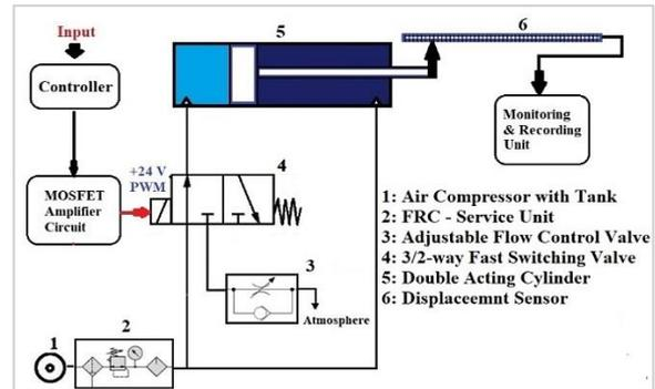
**Figure 2.** The Proposed electro-pneumatic circuit
