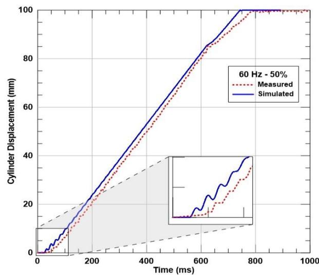
**Figure 3.** Cylinder response to 60 Hz plain PWM valve control signal.
