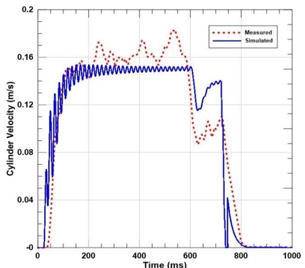
**Figure 4.** Cylinder velocity under the effect of 60 Hz PWM control signal with 50% duty cycle
