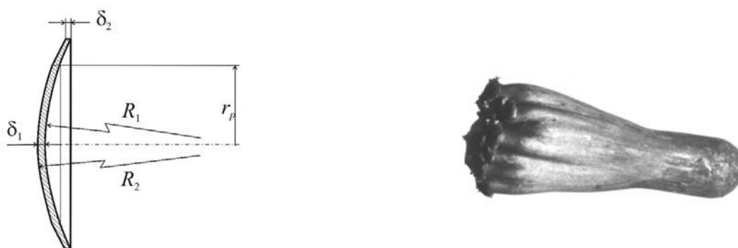
Fig. 1. Spheroconic cumulative cladding Fig. 2. The shape of the elongated high-speed element [1]:
