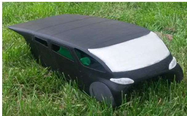
Figure 1. RP in-scale model of a Solar Car [30].
