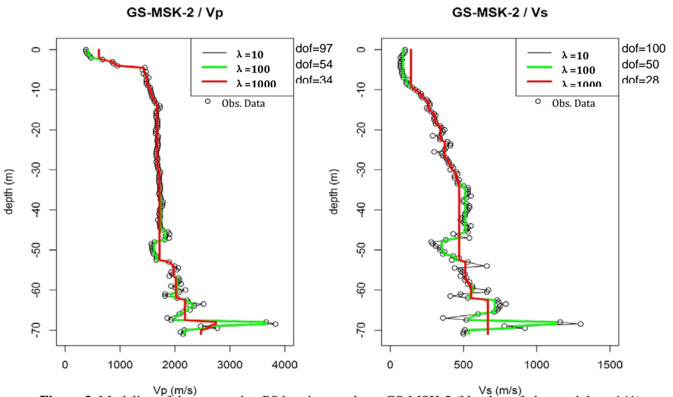
**Figure 3.** Modeling of the suspension PS logging results at GS-MSK-2 (Number of observed data: 141)
