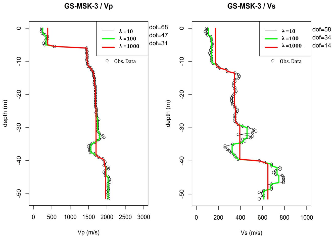
**Figure 4.** Modeling of the suspension PS logging results at GS-MSK-3 (Number of observed data: 103)
