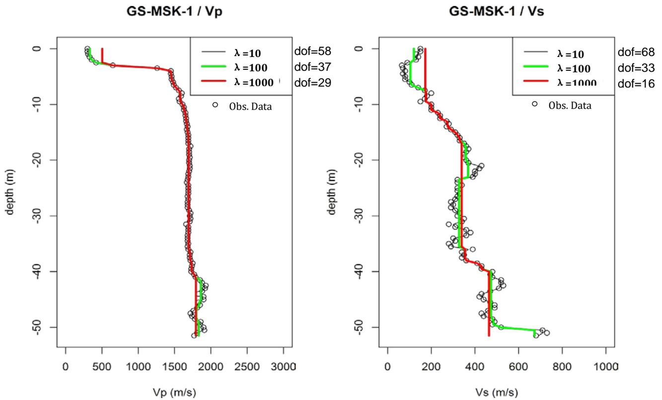
**Figure 2.** Modeling of the suspension PS logging results at GS-MSK-1 (Number of observed data: 104)
