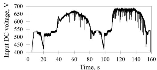
**Figure 5.** The change in input TI with IC voltage during the traction electric drive dynamic testing.
