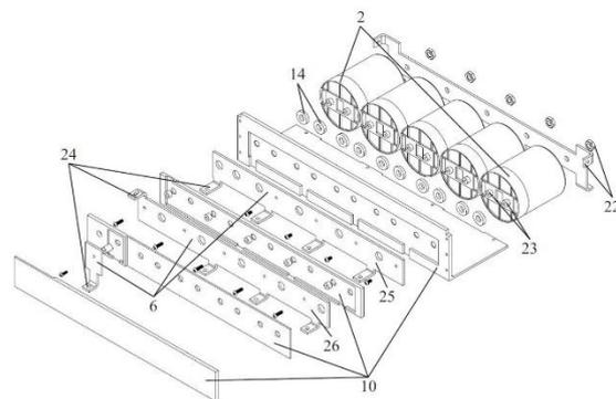
**Figure 3.** The filter capacitor bank with seal elements design and busbar configuration.
