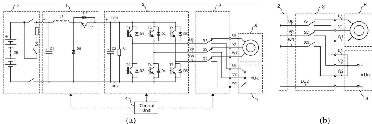
**Figure 1.** Topology of the traction inverter with integrated charger power circuit for use with external (a) three-phase AC and (b) DC voltage source.
