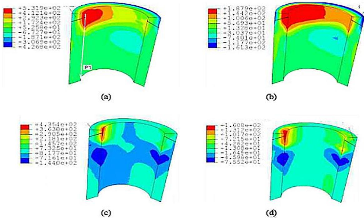
(a) Axial welding stress of welded inner wall; (b) Axis of inner wall after heat treatment; (c) circumferential welding stress of welded inner wall; (d) Circumferential welding stress of inner wall after heat treatment
