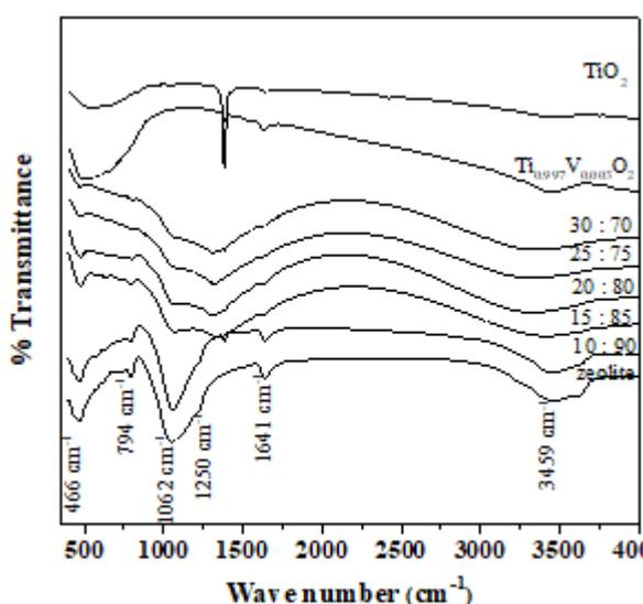
**Figure 3.** FTIR spectra of mordenite zeolite,  $\text{TiO}_2$ ,  $\text{Ti}_{0.997}\text{V}_{0.003}\text{O}_2$ , and  $\text{Ti}_{0.997}\text{V}_{0.003}\text{O}_2/\text{zeolite}$  at various composition.
