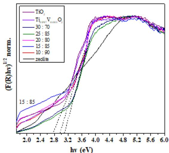
**Figure 7.** Bandgap energy of mordenite zeolite,  $\text{TiO}_2$ ,  $\text{Ti}_{0.997}\text{V}_{0.003}\text{O}_2$ , and  $\text{Ti}_{0.997}\text{V}_{0.003}\text{O}_2/\text{zeolite}$  at various composition
