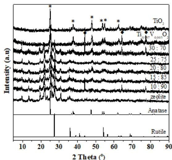
**Figure 2.** XRD pattern of mordenite zeolite,  $\text{TiO}_2$ ,  $\text{Ti}_{0.997}\text{V}_{0.003}\text{O}_2$ , and  $\text{Ti}_{0.997}\text{V}_{0.003}\text{O}_2/\text{zeolite}$  at various composition.
