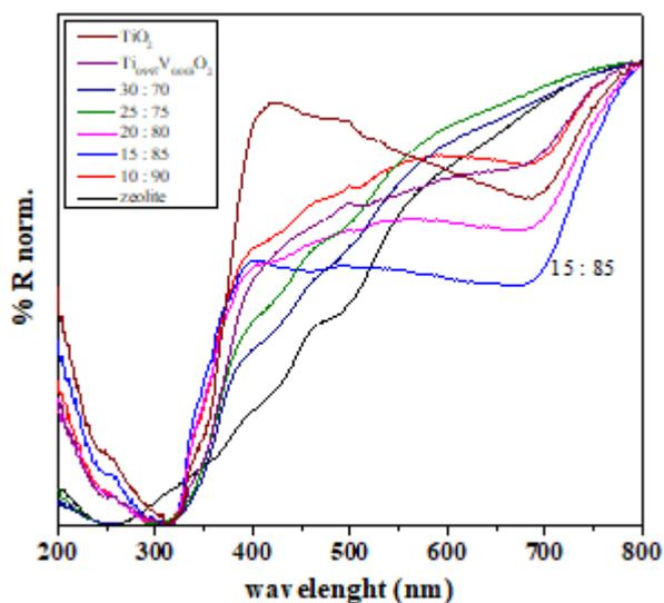
**Figure 5.** Reflectance spectra of mordenite zeolite, TiO<sub>2</sub>, Ti<sub>0.997</sub>V<sub>0.003</sub>O<sub>2</sub>, and Ti<sub>0.997</sub>V<sub>0.003</sub>O<sub>2</sub>/zeolite at various composition.
