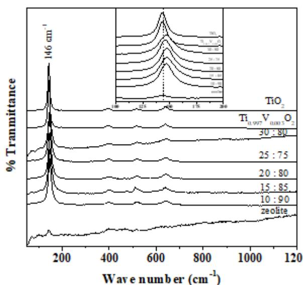
**Figure 4.** Raman spectra of mordenite zeolite,  $\text{TiO}_2$ ,  $\text{Ti}_{0.997}\text{V}_{0.003}\text{O}_2$ , and  $\text{Ti}_{0.997}\text{V}_{0.003}\text{O}_2/\text{zeolite}$  at various composition.
