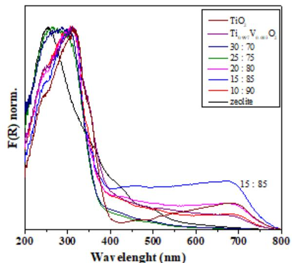
**Figure 6.** Kubelka-Munk function of mordenite zeolite, TiO<sub>2</sub>, Ti<sub>0.997</sub>V<sub>0.003</sub>O<sub>2</sub>, and Ti<sub>0.997</sub>V<sub>0.003</sub>O<sub>2</sub>/zeolite at various composition.
