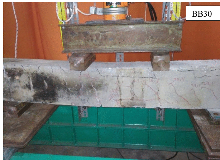
Figure 4. Flexural testing on RC beam BB30 model.
