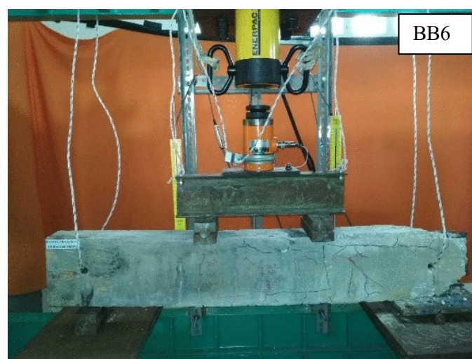
Figure 5. Flexural testing on RC beam BB60 model.
