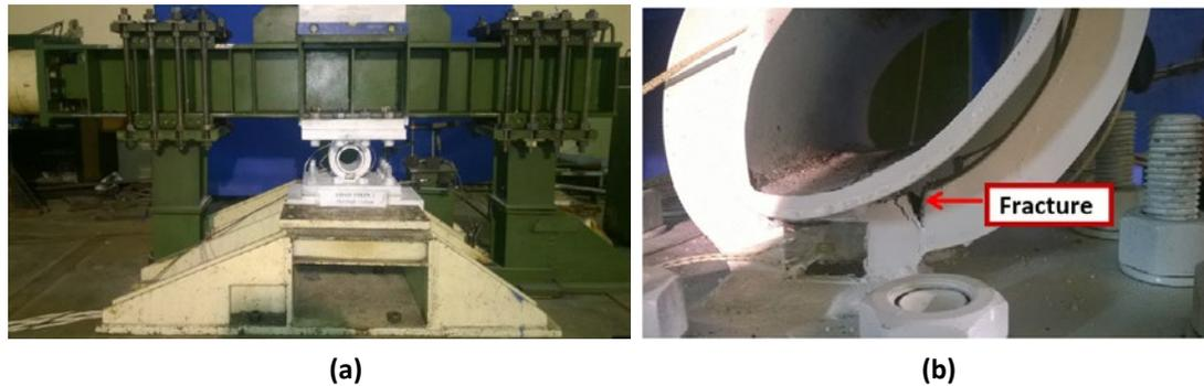
**Figure 7.** Setup specimen for combined rings and horizontal steel pipe damper: (a) Mounting beam for testing specimens and (b) Fracture at point of high intense stress in the tested specimen.
