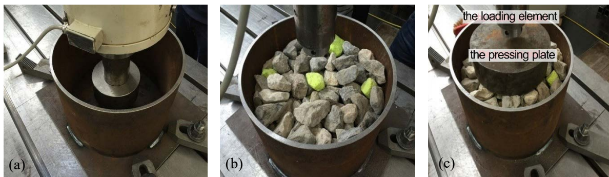
Figure 1. The box test setup (a) the empty cylinder (b) without the pressing plate (c) with the pressing plate.
