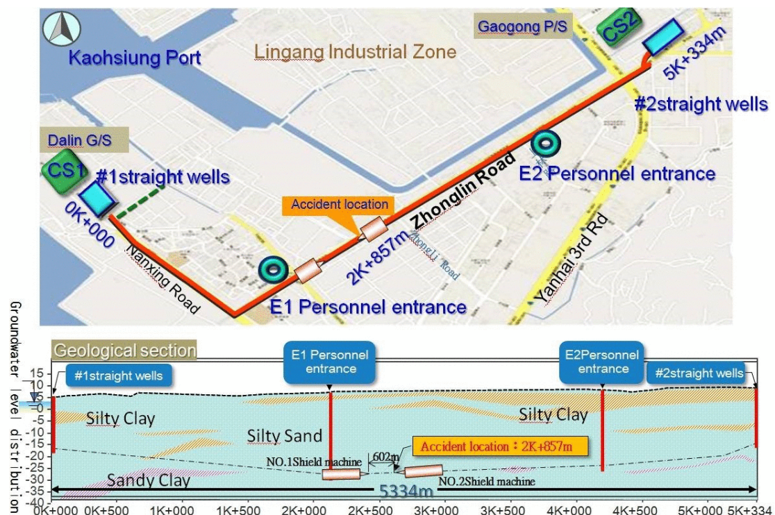
Figure 1. Plan illustration and stratigraphic section of the accident location.
