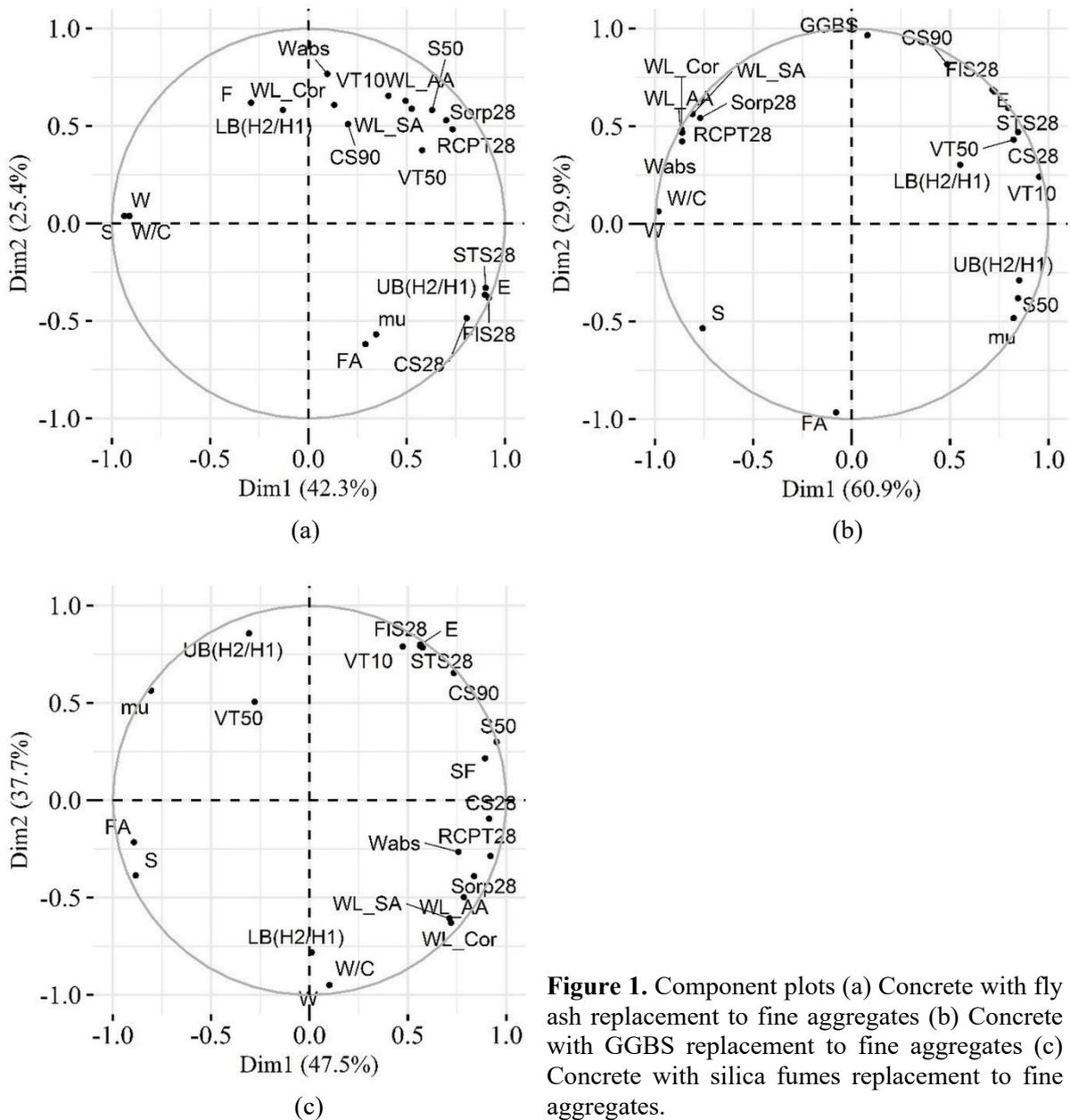
**Figure 1.** Component plots (a) Concrete with fly ash replacement to fine aggregates (b) Concrete with GGBS replacement to fine aggregates (c) Concrete with silica fumes replacement to fine aggregates.
