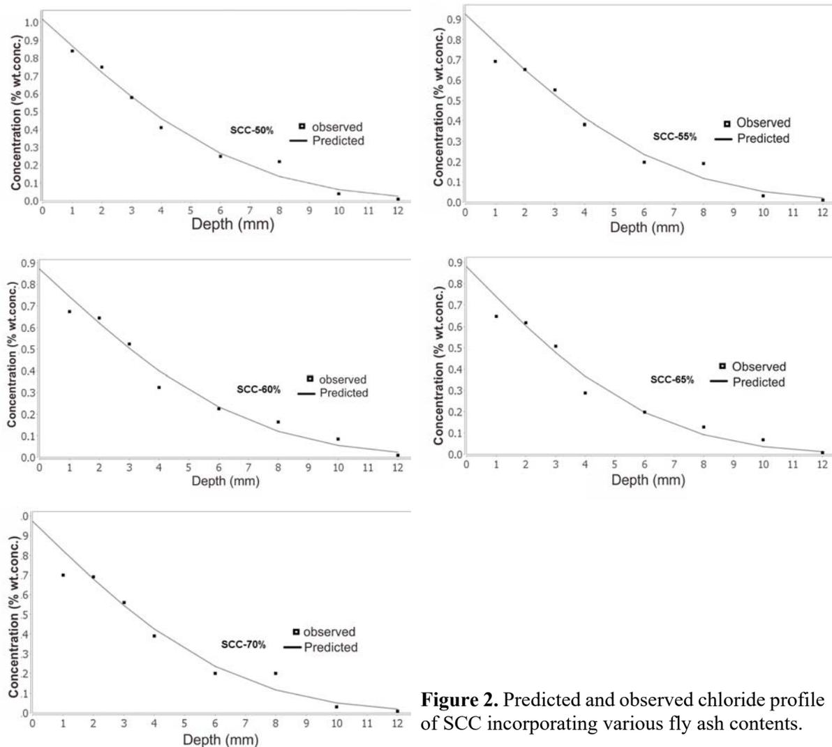
**Figure 2.** Predicted and observed chloride profile of SCC incorporating various fly ash contents.
