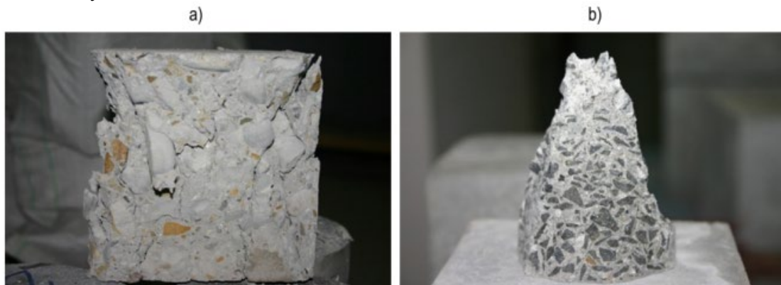
Figure 4. A view of a destroyed concrete specimen: a) normal concrete - the destruction of the matrix with simultaneous maintenance of aggregate grains, b) high-performance concrete – the destruction of the matrix and aggregate grains
