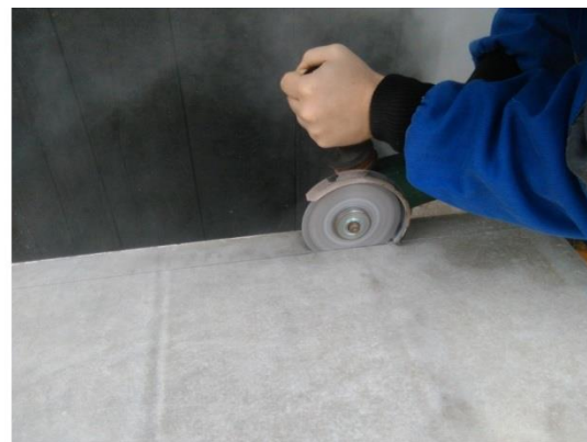
Figure 6. TRC slabs: left – bigger slab; right – cutting of the slab on the specimens.
