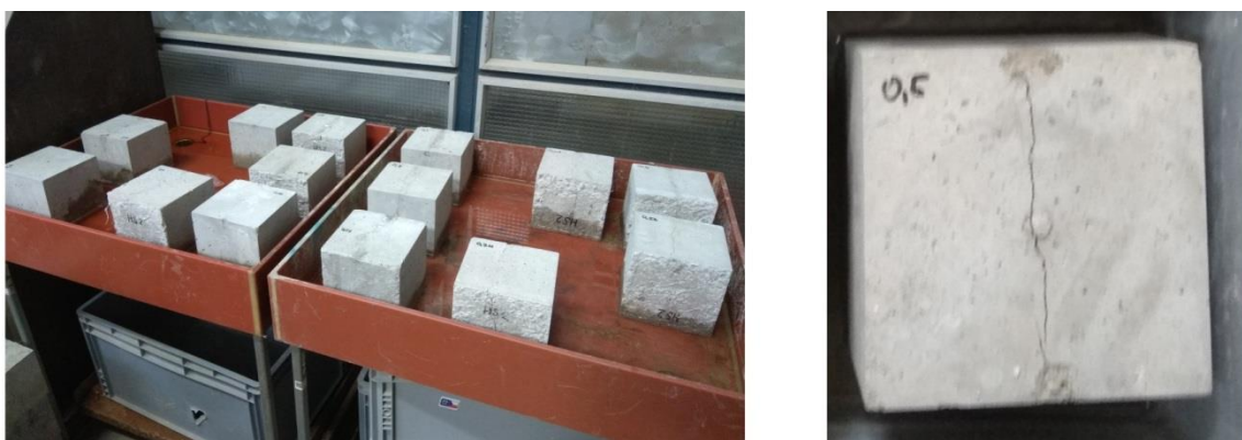
Figure 3. Cube specimens: left – storage of the specimens during the experiment; right – crack in the specimen, width of the crack is about 0.5 mm.
