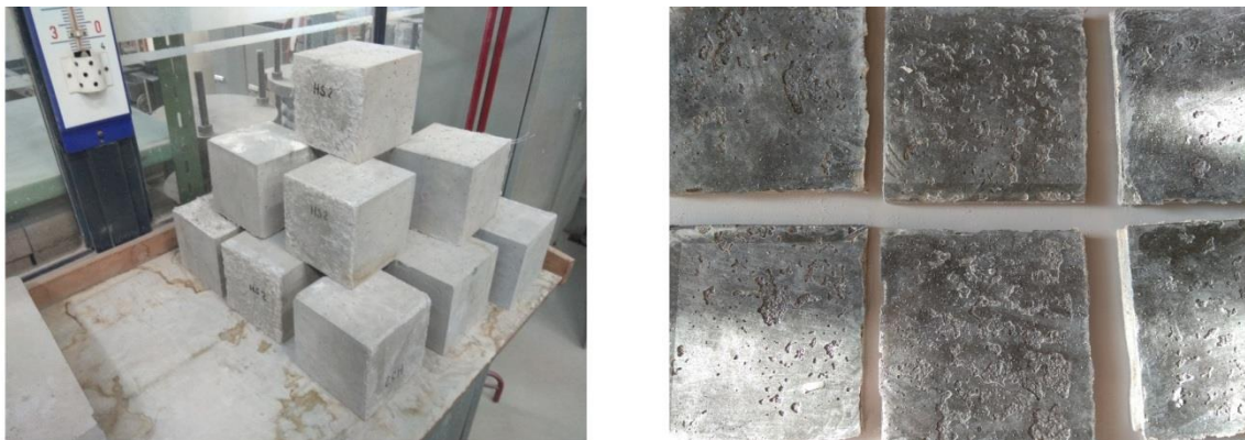
Figure 2. Test specimens: left – cube specimens; right – TRC specimens.
