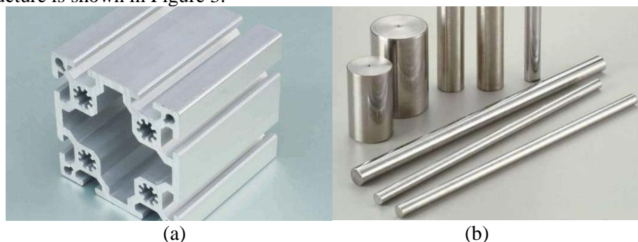
Figure 2. Different structures of aluminum alloy; (a) aluminum alloy sections and (b) aluminum alloy bars.
