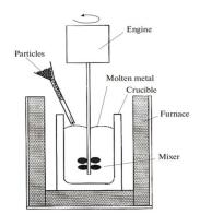
Figure 1. Schematics of mechanical mixing of
