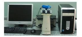
**Figure 3.** Light optical microscope (LECO LX 31) connect with camera (Pax cam) to image analysis software (Pax-it).
