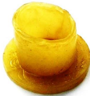
Figure 3. The resulting product at a temperature of 155°C injection
