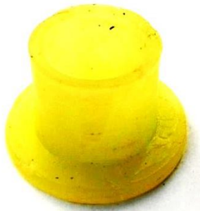
Figure 5. The resulting product at a temperature of 165 °C
