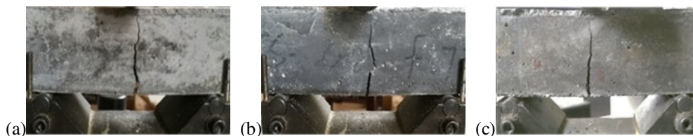
Figure 5. Failure modes of the non-fiber high performance concrete specimens with different copper slag replacement rate in the bending tests. (a) 0%; (b) 40%; (c) 100%.
