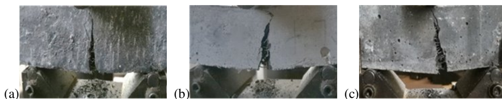
Figure 6. Failure modes of the steel fiber high performance concrete specimens with different copper slag replacement percentage in the bending tests. (a) 0%; (b) 40%; (c) 100%.
