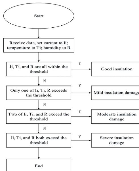
**Figure 3.** Insulation status diagnostic subroutine flow chart
