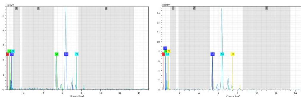
**Figure 4.** EDS spectrum of cleaned stainless steel surfaces and SHSSS (a) cleaned stainless steel surface (b) SHSSS
