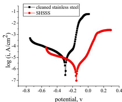
**Figure 7.** Tafel polarization curves of cleaned stainless steels surface and SHSSS in 3.5 wt% NaCl solution
