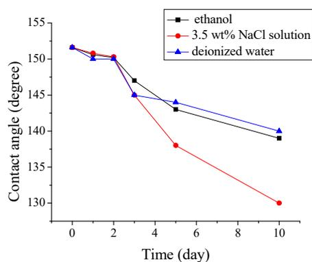
**Figure 5.** The change curve of WCAs of SHSSS with the increase of soak time in different solutions
