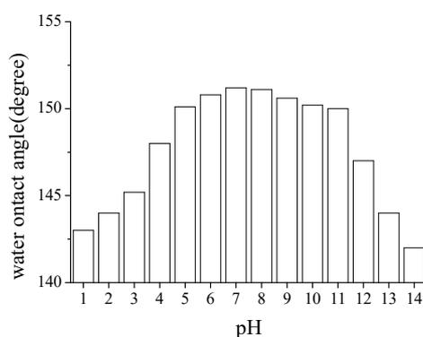
**Figure 6.** WCA of SHSSS after soaking in solution with different pH for 24h
