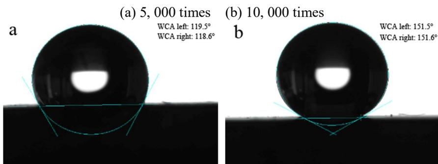
**Figure 2.** WCA image of cleaned stainless steel surface and SHSSS (a) cleaned stainless steel surface (b) SHSSS
