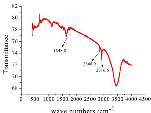
**Figure 3.** FTIR spectrum of modified stainless-steel powder
