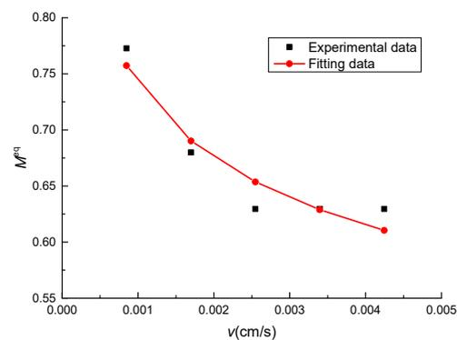
**Fig. 1** Relationship between reaction rate and liquid velocity
