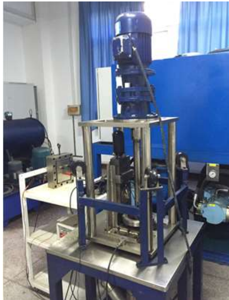
Fig. 8 Test equipment for inclination correction hydraulic system performance simulation
