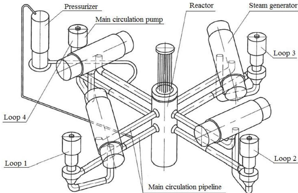
**Figure 1.** The overview diagram of main circulation pipeline.
