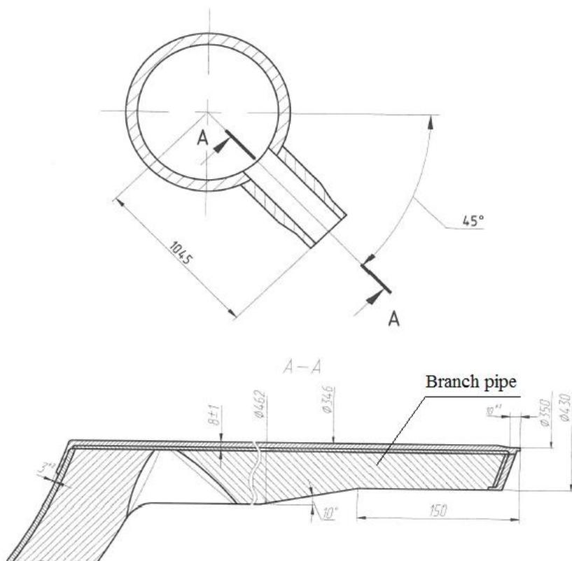
**Figure 2.** The section sketch of DN 350 branch pipe cutting-in in the main circulation pipeline.
