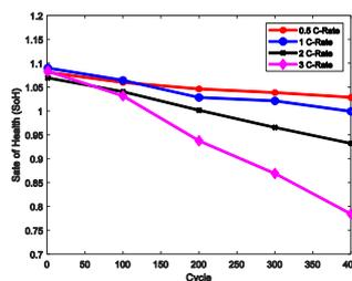
**Figure 5** SoH of LiFePO<sub>4</sub> batteries at 20°C under different C-Rates with 400 cycles.
