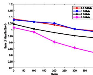
**Figure 6** SoH of LiFePO<sub>4</sub> batteries at 30°C under different C-Rates with 400 cycles.
