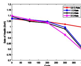
**Figure 8** SoH of LiFePO<sub>4</sub> batteries at 50°C under different C-Rates with 400 cycles.
