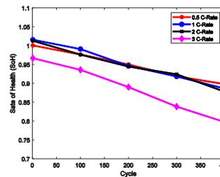
**Figure 4** SoH of LiFePO<sub>4</sub> batteries at 10°C under different C-Rates with 400 cycles.
