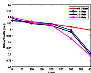
**Figure 7** SoH of LiFePO<sub>4</sub> batteries at 40°C under different C-Rates with 400 cycles.
