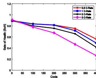
**Figure 2** SoH of LiFePO<sub>4</sub> batteries at -10°C under different C-Rates with 400 cycles.
