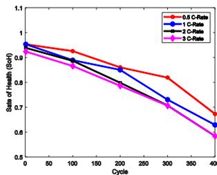
**Figure 3** SoH of LiFePO<sub>4</sub> batteries at 0°C under different C-Rates with 400 cycles.
