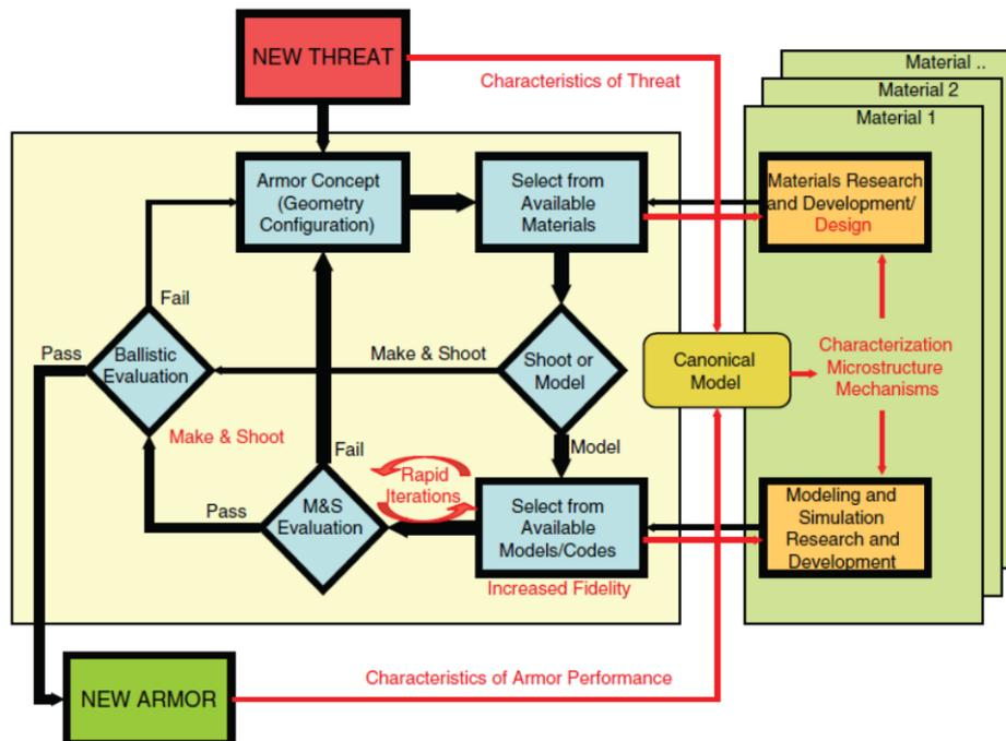
**Figure 3.** Flow chart for (re-)designing an armor [26]
