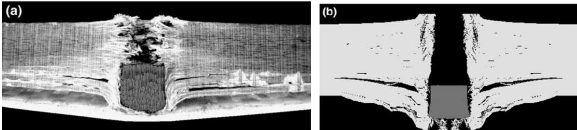
**Figure 6.** Experimental (a) and computational (b) results for an impact of 0.50 caliber FSP with a 25.4 mm, E-glass fiber reinforced poly-vinylester-epoxy matrix. Initial projectile velocity, 605 m/s [32]
