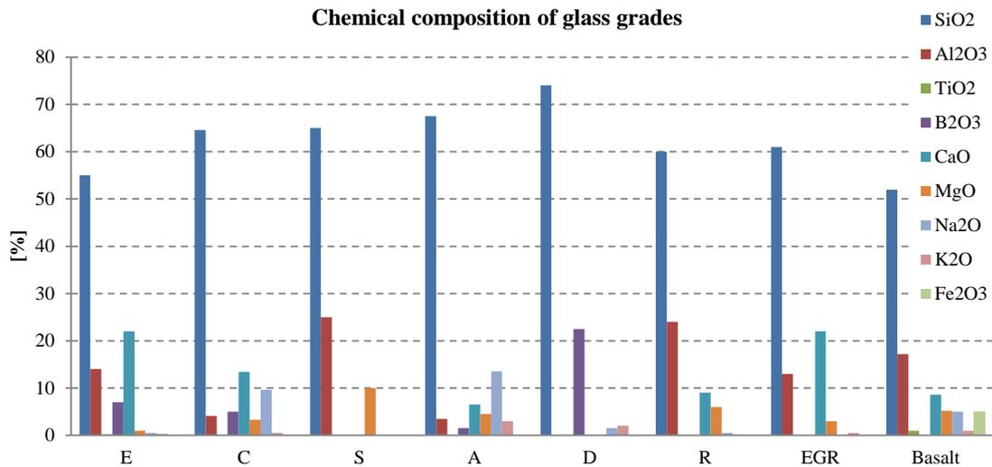
**Figure 1.** Chemical composition of glass grades: A - durability, high mechanical strength and high electric resistivity, C - high corrosion resistance, D - low dielectric constant, E - high mechanical strength and high electric resistivity, AR - alkali corrosion resistance, R- high strength and acid corrosion resistance S - highest tensile strength, S2- high strength, elasticity modulus and stability [5]
