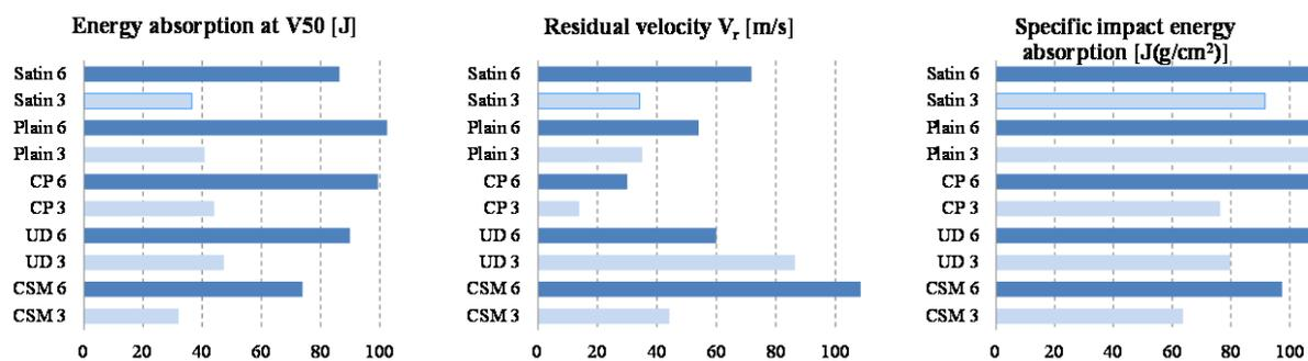
**Figure 9.** Characteristics of several panels obtained with different types of glass fiber and the same matrix: CSM - randomly oriented glass chopped strand of  $400 \text{ g/m}^2$ , UD - unidirectional fabric of  $300 \text{ g/m}^2$ , CP - cross ply laminate,  $[0^\circ, 90^\circ]$  with unidirectional fibers, Plain - a plain-woven roving cloth of  $400 \text{ g/m}^2$ , Satin - a satin cloth of  $300 \text{ g/m}^2$ , 3 - 3 mm thickness, 6 - 6 mm thickness [38]
