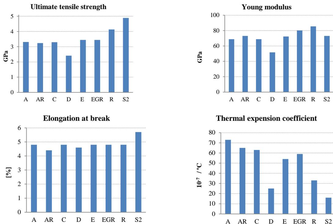
**Figure 2.** Characteristics of glass fibers (after [5])
