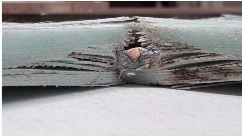
**Figure 7.** Composite glass fiber + resin, thickness of 13 mm, after the impact with 9 mm FMJ at 420 m/s [34]
