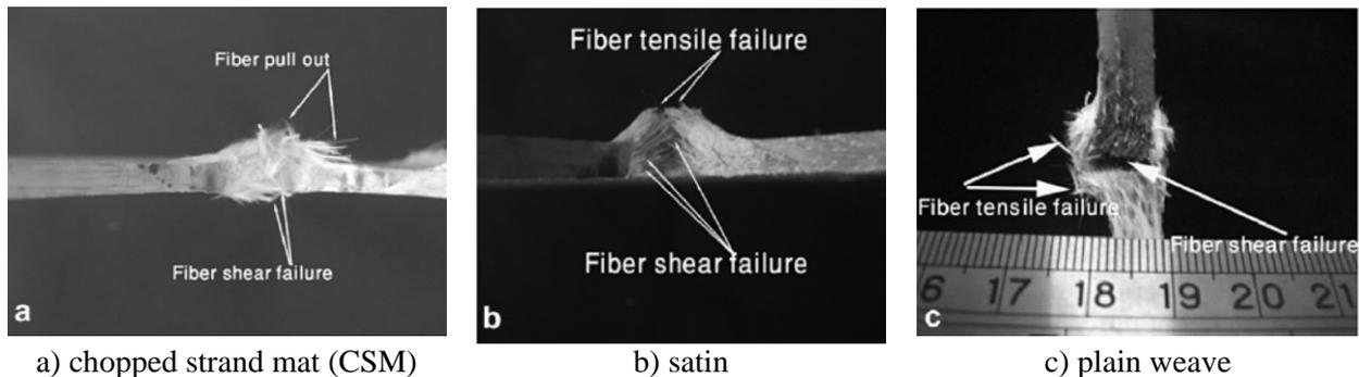
**Figure 10.** Quarter section of 3 mm thin-walled reinforced samples (95 m/s) [38]
