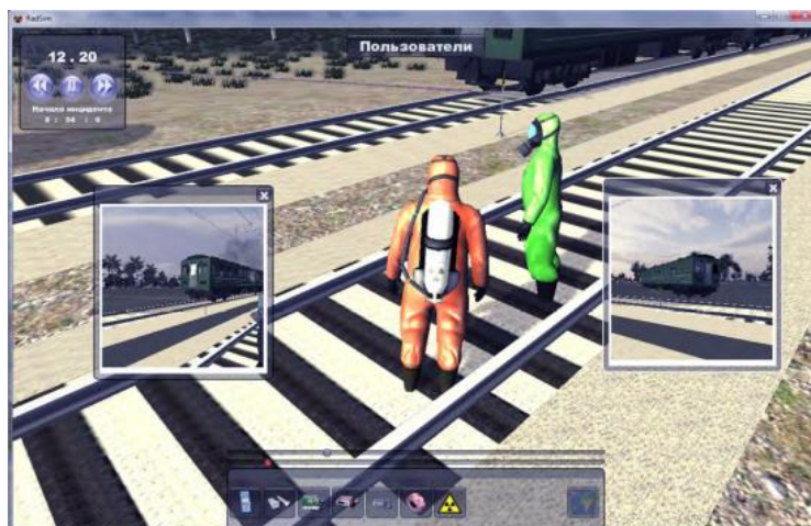
Figure 1. Three-dimensional simulator for training the actions of personnel of rescue units for the detection of radioactive contamination and the conduct of radiation reconnaissance
