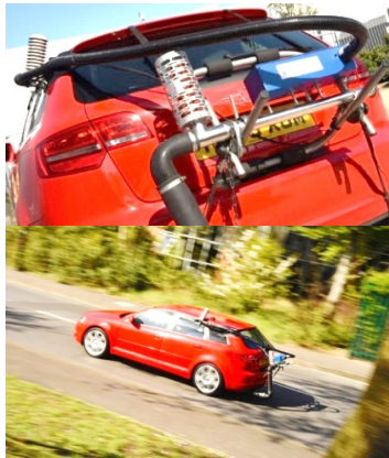
Figure 11. Portable emissions testing systems used by independent EQUA Air Quality Index, powered by Emissions Analytics, April 2016 (source: https://equaindex.com/ )
