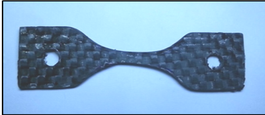
Figure 3. Final shape of creep specimen according to the ASTM-D2990.
