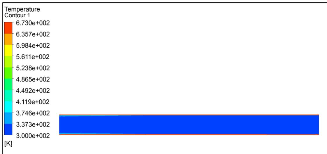
**Figure 6.** Temperature distribution for smooth circular passage.
