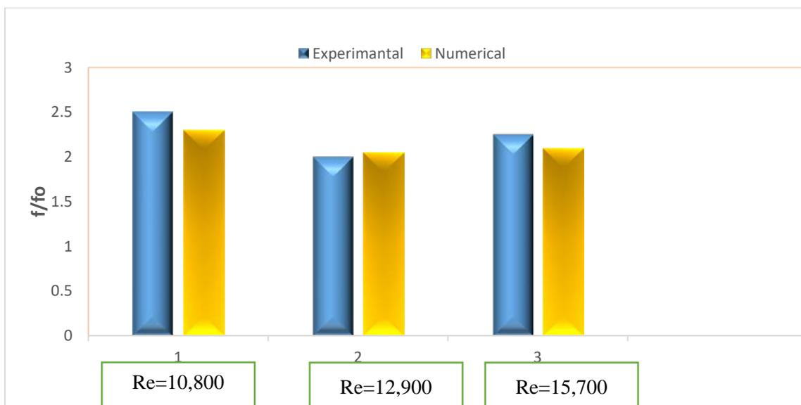
**Figure 13** Experimental and numerical comparison of friction factor ratios with varying Reynolds numbers
