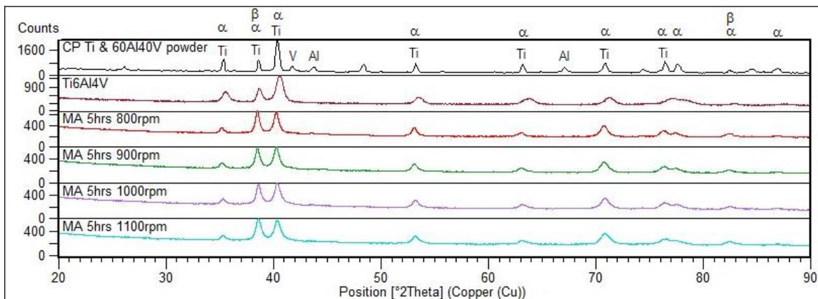
**Figure 4.** XRD results of the (a) CP Ti and 60Al40V powder, (b) standard Ti6Al4V alloy and mechanically alloyed CP Ti and master alloy for 5 hours at different speeds of (c) 800 rpm, (d) 900 rpm, (e) 1000 rpm and (f) 1100 rpm.
