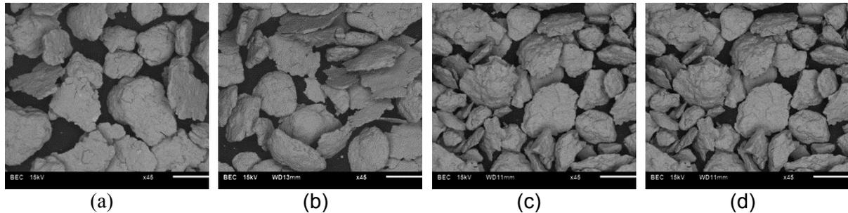
**Figure 2.** SEM micrographs after milling Ti and master alloy at a constant ball to powder ratio (20:1), milling duration (5 hours) and different speeds of (a) 600rpm, (b) 800rpm, (c) 1000 rpm and (d) 1100rpm.
