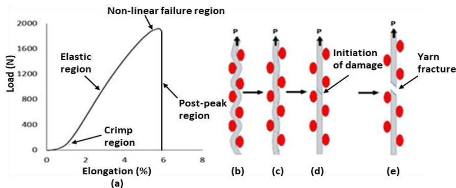
**Figure 3.** (a) Load-elongation curve during tensile loading, (b) crimp region, (c) elastic region, (d) non-linear failure region and (e) post-peak region (adapted and reproduced) [10]
