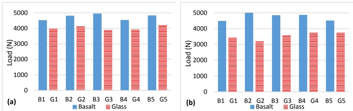
**Figure 8.** Peak load of Basalt and Glass woven fabric samples along (a) weft and (b) warp
