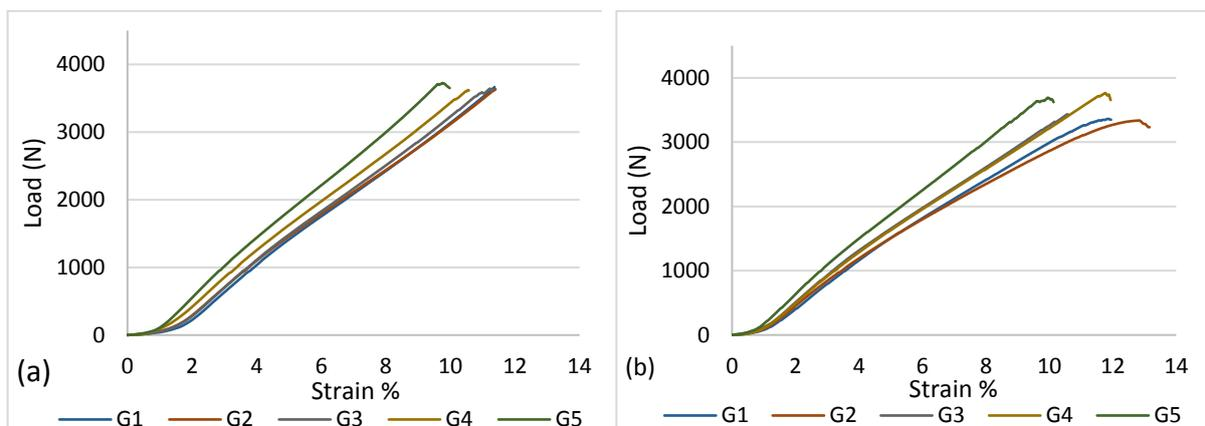
**Figure 5.** Average Load vs elongation curves for Glass fabrics along (a) weft and (b) warp.
