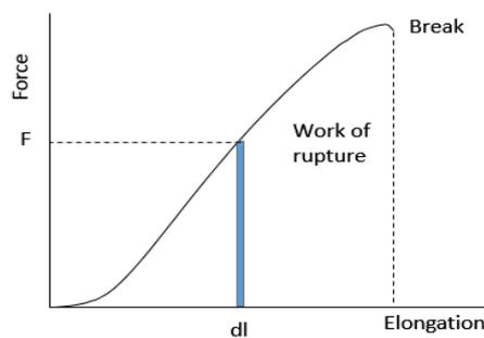
**Figure 6.** Work of rupture in force extension curve
