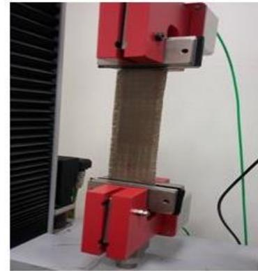
Figure 2. Tensile testing of sample fabrics
