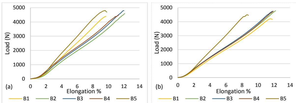
**Figure 4.** Average Load vs elongation curves for Basalt fabrics along (a) weft and (b) warp.
