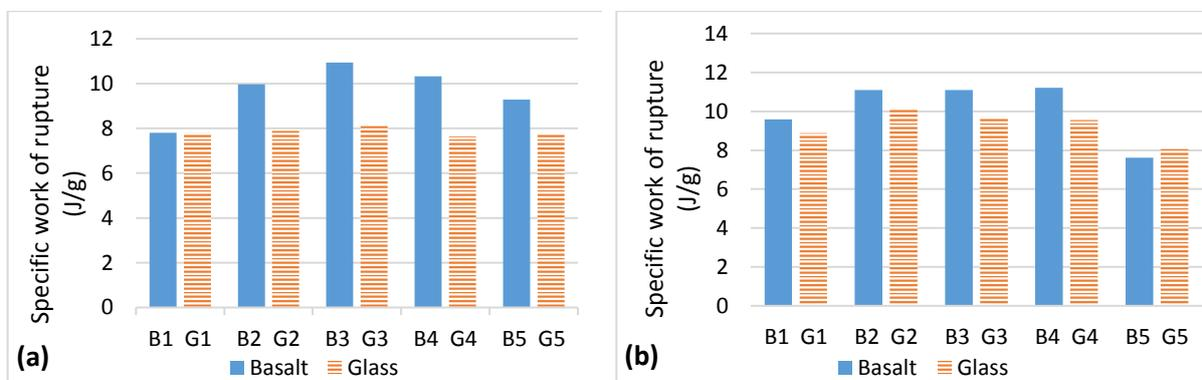
**Figure 7.** Specific work of rupture for Basalt and Glass woven fabrics along (a) weft and (b) warp
