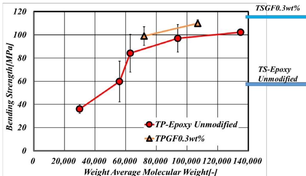
**Figure 8.** Relationship between bending strength and weight-average molecular weight on epoxy resin plate.
