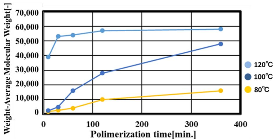
**Figure 3.** Relationship between Mw and polymerization time on temperature.
