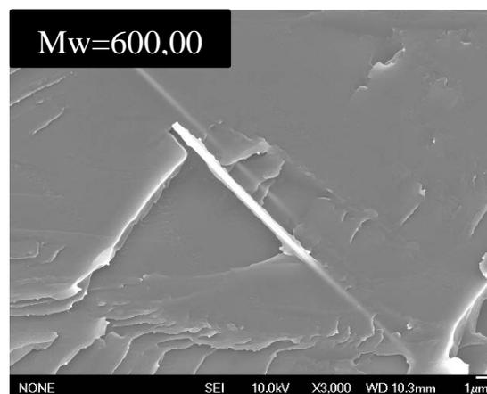
**Figure 11.** State of the fracture surface on addition of glass fiber on thermoplastic epoxy.
