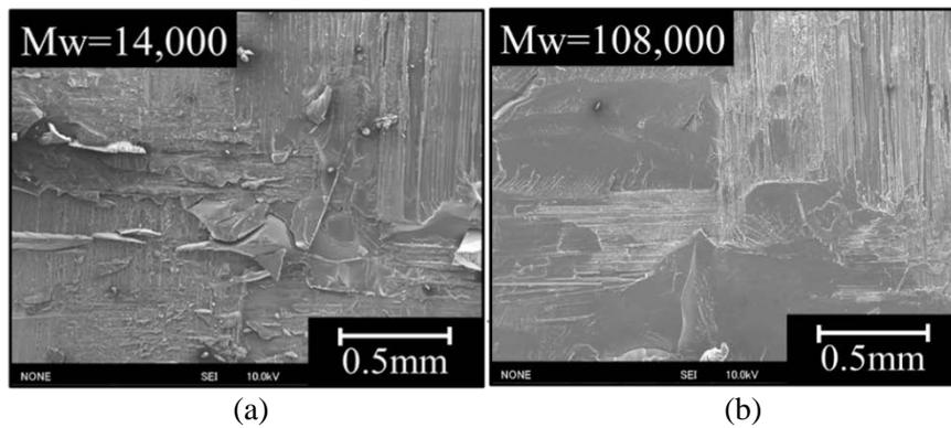
**Figure 10.** State of the fracture surface for Mw: (a) 14,000 and (b) 108,000.
