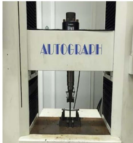
**Figure 6.** Test device for bending test.
