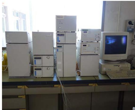
**Figure 4.** Measuring equipment of weight average molecular weight of resin. (Gel Permeation Chromatography; GPC)
