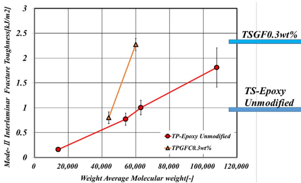
**Figure 9.** Relationship between Mode- II interlaminar fracture toughness and weight-average molecular weight and addition of glass fiber.
