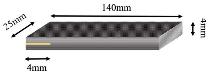
**Figure 7.** Geometry of ENF specimen.
