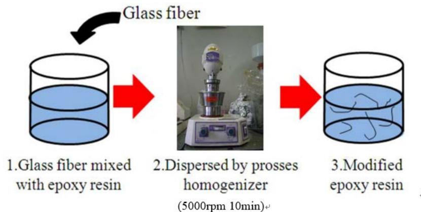
**Figure 5.** Mixed glass fibers with epoxy resin.
