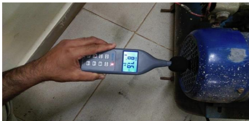
Figure 7. Noise test on the motor with good Bearing.
