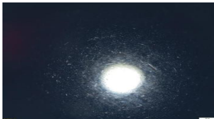
Figure 5. Ball of good Bearing under microscope (5X magnification).
