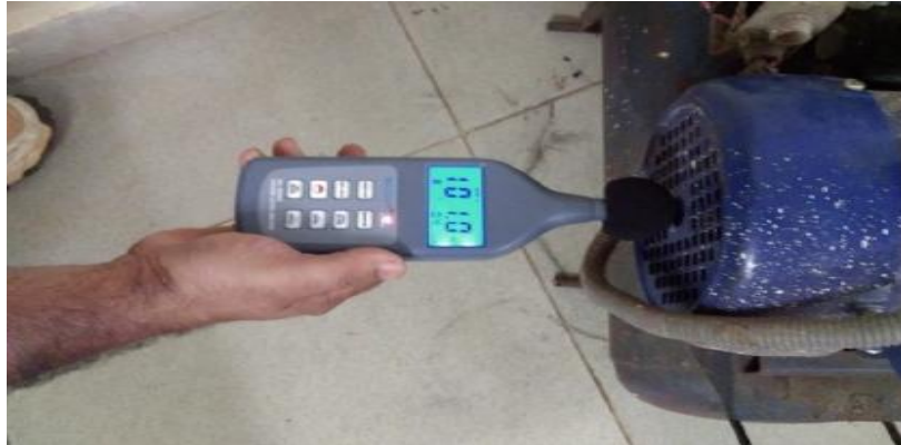
Figure 6. Noise test on the motor with Damaged Bearing.
