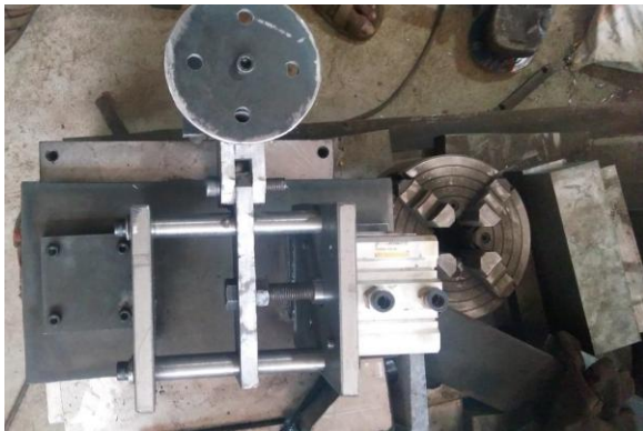
Figure 9. Fabricated Model of the fixture.
