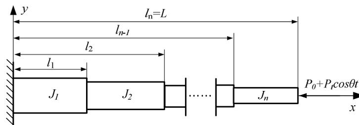
**Figure 1.** The mechanical model of dynamic stability for multi sectioned telescopic boom.
