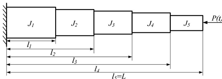
**Figure 2.** The calculation model of 5-section telescopic boom.
