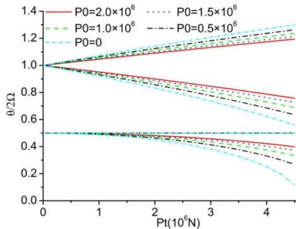
**Figure 3.** Dynamic curves of clamped 5-sections stepped column under different axial resonant forces.
