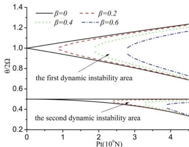
**Figure 4.** Parametric vibration curves of telescopic boom with different damping coefficients.
