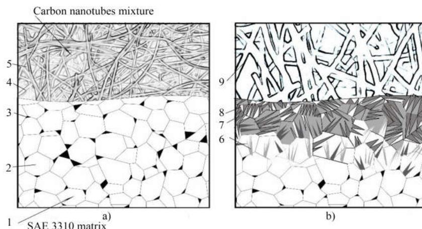
**Figure 3.** Carburized layer mechanism a) at starting time b) absorption of carbon atoms (1-steel structure; 2-ferrite; 3-pearlite; 4-carbon nanotubes; 5-emulsion; 6-cementite; 7- martensite; 8- austenite; 9-carbon nanotubes).
